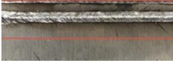
Consistent topbead, no spatter or blowholes
