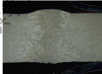
6mm, butt joint, 2.0m/min, 2.0kW+1.5kW
